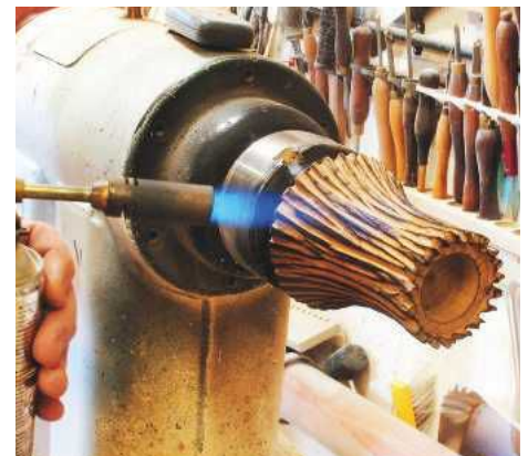
▲ Pic.12 The best way of removing any rough areas left after the texturing is with the blow torch but do remove any shavings or dust around the lathe
